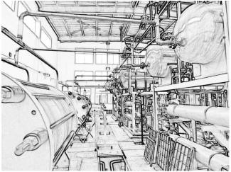
hydrogen and oxygen separators, there hydrogen and oxygen are separated with electrolyte due to gravity. Hydrogen and oxygen gases are allowed to pass through hydrogen and oxygen coolers separately and are cooled to the temperature of 30~40°C.
